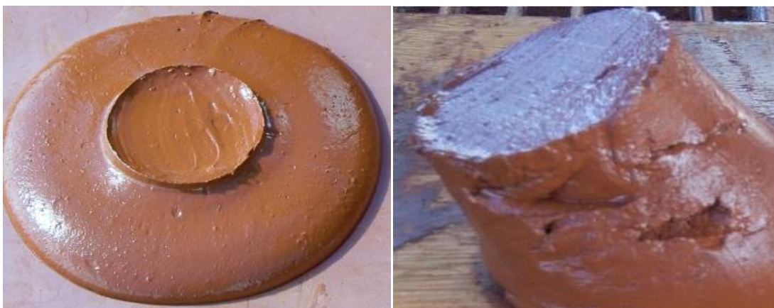
Figure 7. Alumina refinery plant trial with Jamaican bauxite residue that encompassed utilization of a bauxite with a high goethite concentration; slump of untreated bauxite residue (left) and treated bauxite residue (right)
